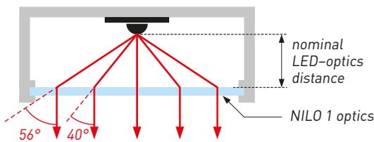
It is important to realize that it is essentially the light bending power that is fixed (in the figure, it is “bent by 40°” or “bent by 56°”). Thus, when the incoming light is changed, the outgoing light changes as well.
