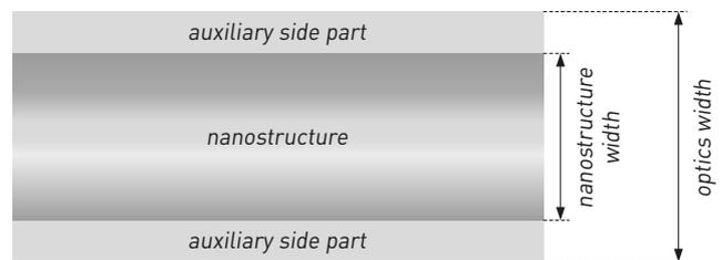
Width may be also affected when using optics in off-axis position. For instance, if one wants to use a fixture with centrally positioned LEDs and NILO 1 optics with decentering offset 5 mm, the maximum width of optics is just 30 mm.
