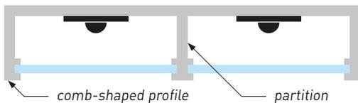
It might be especially advantageous to ask for a custom IQ Linear with several optics next to each other on a single substrate. In that case, partitions between individual rows might not be necessary if crosstalk between rows is negligible. However, partitions may still be useful for supporting the optics.
