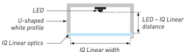
Such luminaire construction is used to measure the nominal parameters, e.g., beam width (FWHM), peak luminous intensity, etc. One parameter deserves special attention: the specific efficiency. As efficiency of the luminaire depends a lot on, e.g., particular white material of the fixture, a real efficiency (flux of luminaire / flux of LED) would be misleading. Thus, the spe-
