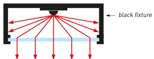
A luminaire with diffused white surface behaves differently. Light that hits the fixture surface is now diffusely reflected. Some light is reflected towards the optics and leaves the luminaire. However, such reflected light hits the optics at a random angle and subsequently leaves the luminaire at a random angle too. Light distribution is thus combined with basically omnidirectional light, leading to wider light distributions on more stray light. On the other hand, efficiency of such
