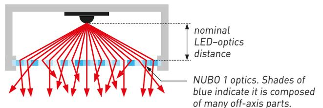
Moreover, those tiny parts are mixed in a way that each small area of IQ Linear tries to create the same light distribution. This enhances homogeneity of the light emitting surface and allows one to adjust IQ Linear width without significantly affecting the optical function.
