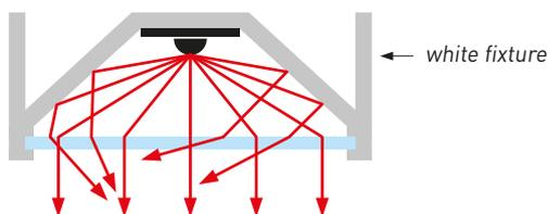
Another way to reduce multiple reflections is to use a glossy or even mirror-like surface. A well designed luminaire interior reflects light just towards the optics, i.e., multiple reflections are avoided. However, a new phenomenon appears: a mirror-like slanted wall creates a mirror image of the LED, i.e., it seems that the optics is illuminated by multiple LEDs at once.
