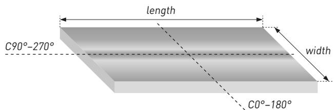
In the direction parallel to the luminaire length ( $C90^\circ$ – $270^\circ$ ), IQ Linear optics does not affect light significantly. To put it in another way, light distribution in  $C90^\circ$ – $270^\circ$  is about the same like light distribution of the LED, i.e., usually FWHM  $120^\circ$ . Such a wide light distribution contributes to glare.
