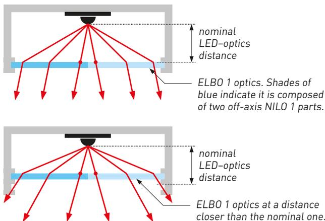
To explain all other IQ Linear types, it is worth reminding that the light bending features are very small. This allows to split the area of the optics not just to two parts like in ELBO 1, but to many more tiny parts, tens or hundreds of them. For instance, the NUBO 1 optics making a batwing light distribution is split to hundreds of tiny parts, each behaving like off-axis NILO 1, each redirecting light to a specific direction. The directions and corresponding amount of light are precisely bal-
