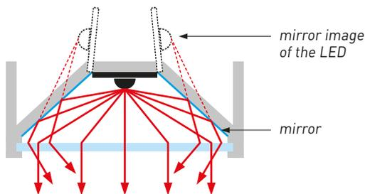
Such a behaviour may be acceptable when creating wide light distributions. Stray light will be reduced compared to white surfaces as light is not randomly scattered. On the other hand, a mirror surface will likely cause problems when creating extremely narrow beams – instead of single narrow beam, several sur-
