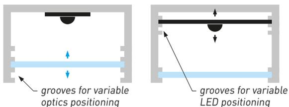
Width of the optics, or more precisely clear aperture width, does not usually affect light distribution significantly. For instance, NILO 1 optics (see page 6) mounted 3 mm from LEDs creates a medium wide beam with FWHM from 49° to 52° for the optics width from 10 to 40 mm. Indeed, wider optics generally lead to more efficient luminaires as more light directly hits the optics.
